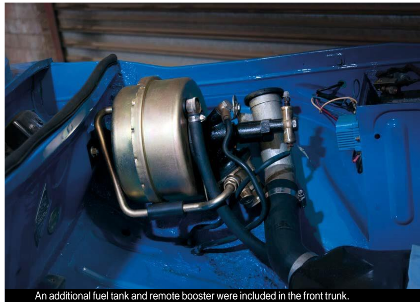
An additional fuel tank and remote booster were included in the front trunk.
