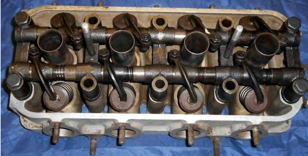
Crossflow cylinder head with twin overhead rocker shafts driven by the single block-mounted camshaft.
